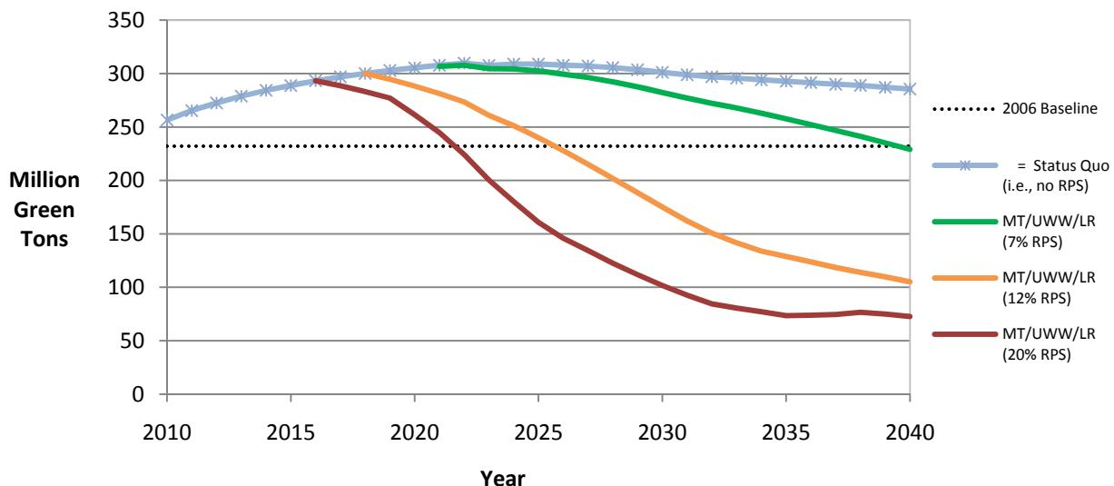
**Figure 6.** The SRTS model-generated pine roundwood inventory. Merchantable timber (MT), urban wood waste (UWW) and logging residue (LR) are used to meet woody biomass demand of a 7%, 12%, or 20% RPS under “base” other renewable energy sources (ORES) assumptions. Also shown are changes in pine roundwood inventory without an RPS mandate and a 2006 baseline.
