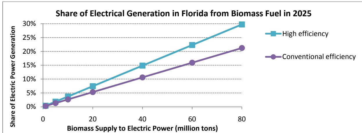
**Figure 2.** Share of electrical power generation in Florida from biomass fuels under conventional (25%) and high (35%) thermal efficiencies at different levels of biomass supply to power plants in 2025.
