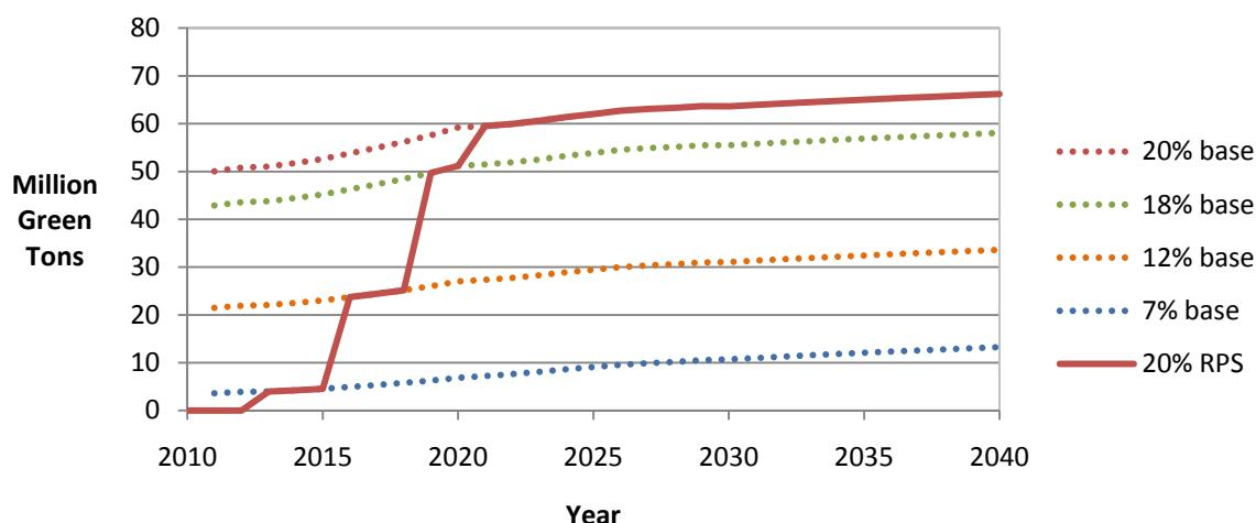
**Figure 1.** Projected change in demand for woody biomass above 2007 harvest levels of 20 million green tons resulting from a theoretical 20% renewable portfolio standard (solid line), assuming “base” other renewable energy sources (ORES) projection and a step-wise portfolio adoption. Also shown projected amount of woody biomass needed for a hypothetical 7%, 12% or 18% RPS with base ORES assumptions.
