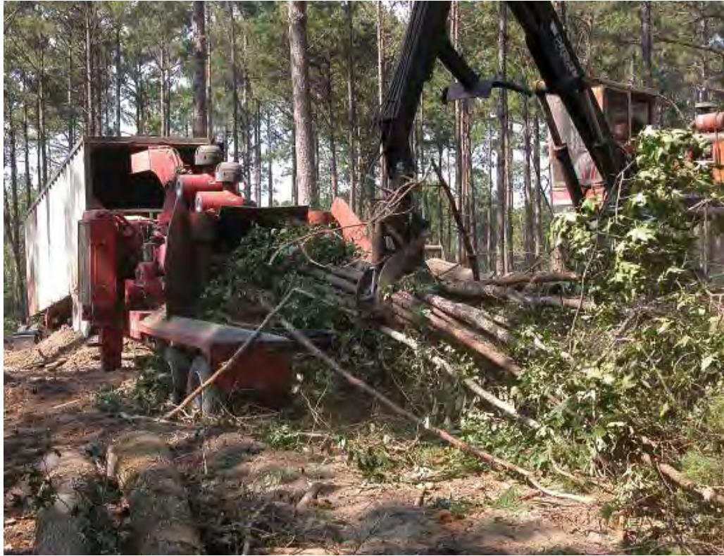
Figure 7: Travis Taylor Logging & Chipping, of Winn Parish, removes understory trees and brush on the Kisatchie National Forest and on private timberlands. Here, the loader (right) feeds whole trees into the chipper (left), which blows the chips into the truck behind it. The chips are utilized for paper and energy at a nearby paper mill.
