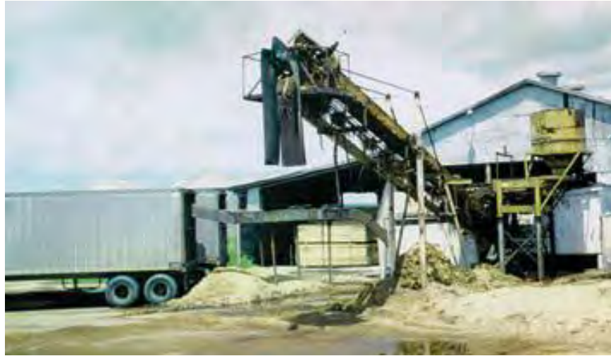
Figure 10: Sawdust, bark and wood trimmings from this hardwood mill are trucked to a paper mill. Some of the material is used to make paper, while the rest is used for energy.
